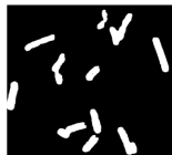
dilation with 3x3 structuring element
