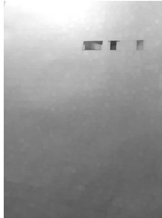
Dilation (local max) 61x61 structuring element
